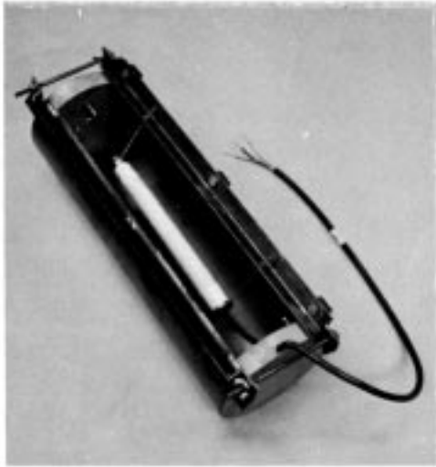
FIG. 1 Horizontal Mold for Creep Specimens
