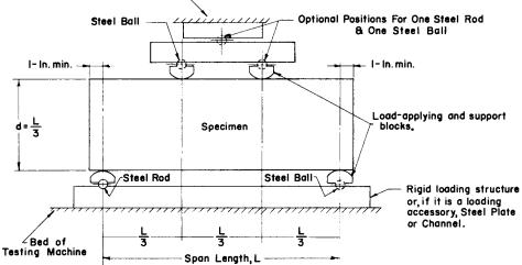
Note 1—This apparatus may be used inverted. If the testing machine applies force through a spherically seated head, the center pivot may be omitted, provided one load-applying block pivots on a rod and the other on a ball. Note 2—1 in. = 25.4 mm.
