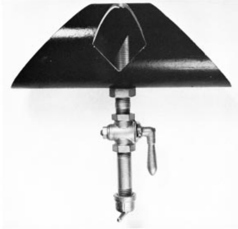
FIG. 5 In-Line Asphalt Sampling Device
