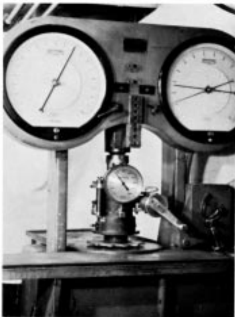
FIG. 3 Hveem Stabilometer Placed in the Testing Machine
