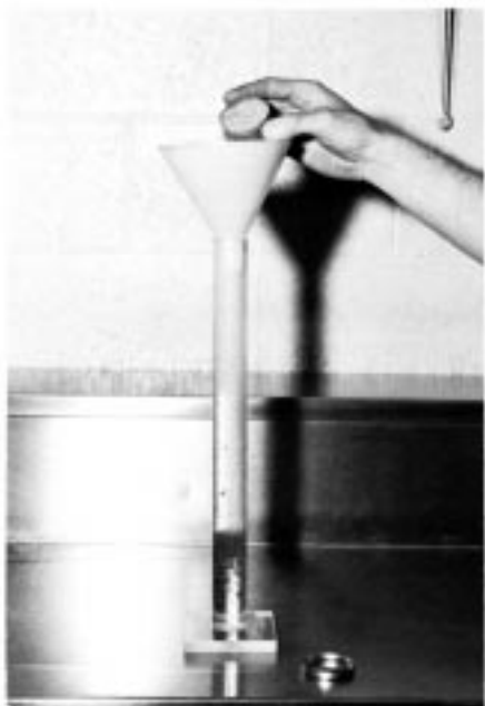
FIG. 5 Transfer of Samples from Measuring Tin to Cylinder
