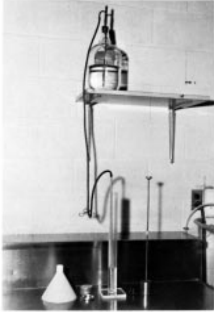
FIG. 4 Graduated Cylinder, Irrigator Tube, Weighted Foot Assembly, and Siphon
