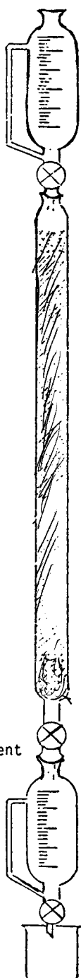
FIG. 1 Chromatographic Column for Separation of Asphalt by Elution-Adsorption (Method A or B)
