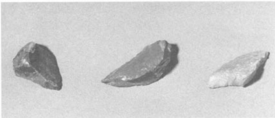
FIG. 3 Fractured Particle (Sharp Edges, Smooth Surfaces)
