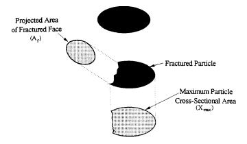
A face will be considered a "Fractured Face" only if it has :  $A_f \ge 0.25 X_{max}$ FIG. 1 Schematic of a Fractured Particle with One Fractured Face
