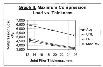
FIG. X3.2 Maximum Compression Load vs. Thickness
