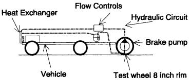
FIG. 2 Sample Brake Systems
