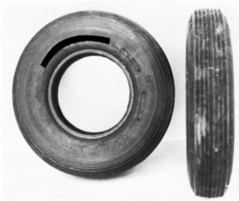
FIG. A1.1 Mu-Meter Test Tire
