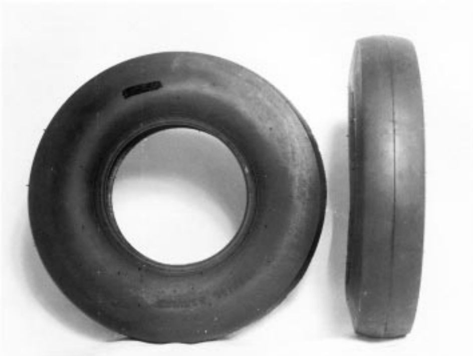
FIG. A2.1 Alternate Mu-Meter Tire
