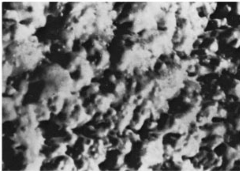
FIG. 5 Polyurethane Foam Texture—Popcorn
