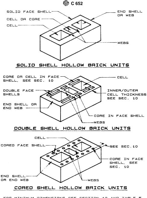
FOR MINIMUM DIMENSIONS SEE SECTION 10 AND TABLE 5 FIG. 1 Hollow Brick Units
