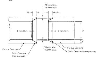
NOTE--See Tables 1 and 2 for values of *D*, *T*, and *L<sub>g</sub>*. FIG. 1 Joint Dimensions
