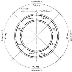
Note 1—The total reinforcement area (Asi) of the inner cage plus the quadrant mat in Quadrants 1 and 2 shall not be less than that specified for the inner cage in Tables 1-5.
