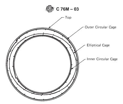
Note 1—The total reinforcement area of the inner circular cage and the elliptical cage shall not be less than that specified for the inner cage in Tables 1-5.
