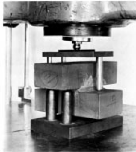
FIG. 6 Crossed-Brick Test Assembly Positioned in Testing Machine
