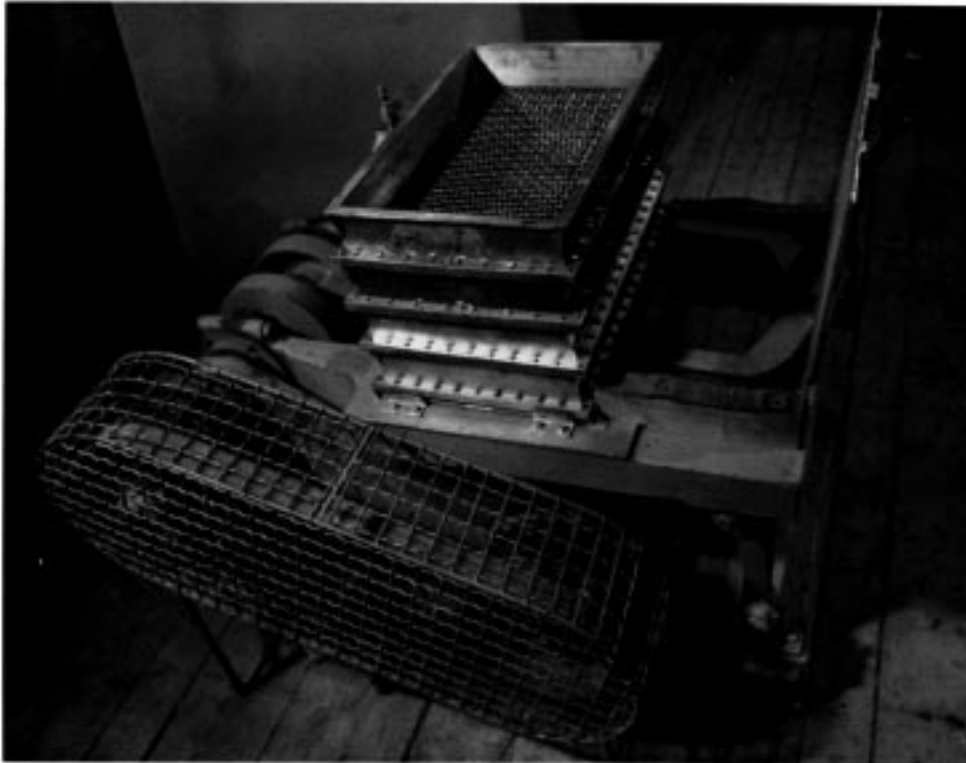
FIG. 1 Quebec Standard Asbestos Testing Machine, Model 2.
