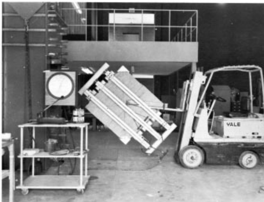
FIG. A1.1 Application of Edge Loads by Clamping a Steel Loading Frame to the Specimen
