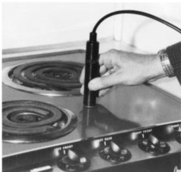
FIG. 3 Applying the Thermesthesiometer to a Horizontal Surface
