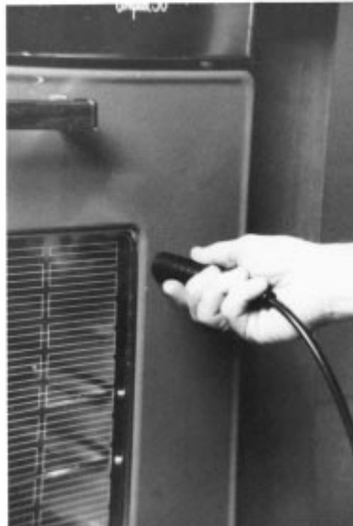
FIG. 4 Applying the Thermesthesiometer to a Vertical Surface
