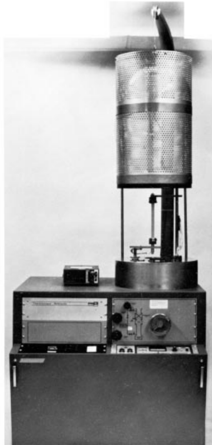
FIG. 3 Example of Vacuum Emittance Test Facility
