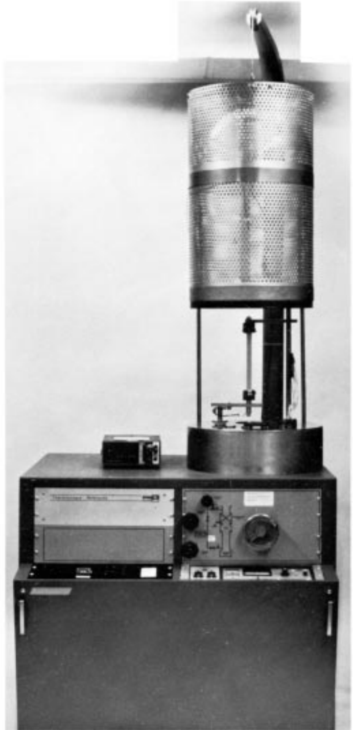
FIG. 3 Example of Vacuum Emittance Test Facility
