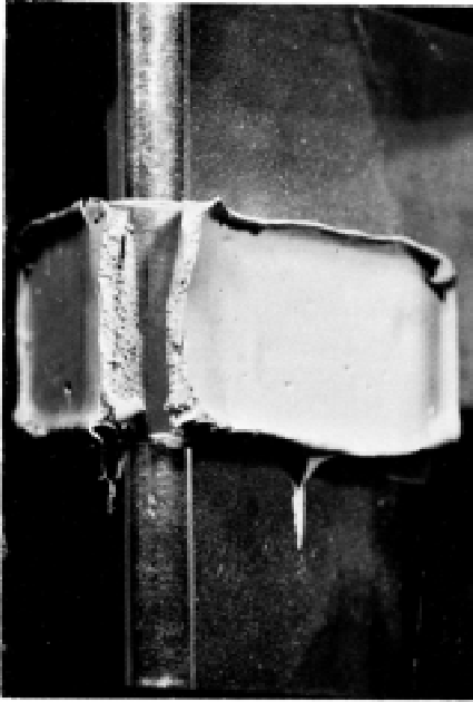
(a) Complete Cracking and Adhesive Failure
