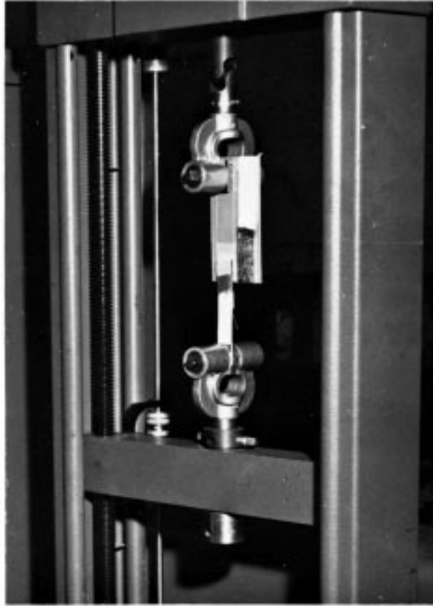
FIG. 2 Extension Machine Used in the Adhesion-in-Peel Test
