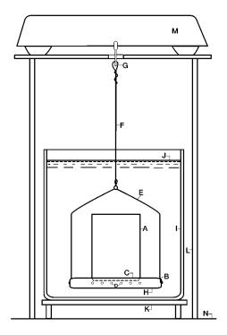
Note 2—The bulk specific gravity gives a convenient and accurate means of calculating the unit weight of the stone; for example, drystone weight per cubic metre (cubic foot) = bulk specific gravity  $\times$  1000 (62.4).
