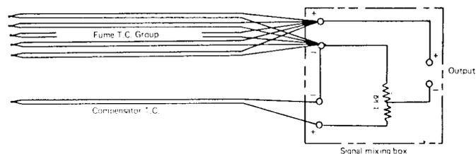
NOTE 1—Two sets of thermocouples and lead wires are required. The wire size and lengths within the fume thermocouple circuit group must be the same to ensure proper signal averaging. The parallel connection of the couples shall be achieved at the mixing box by plug connection of the leads. This allows quick removal and checks for continuity and grounding problems with minimum delay. No cold junction shall be used but the signal mixing box shall be shielded from panel radiation.
