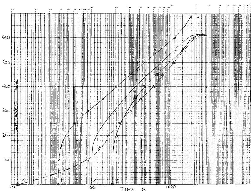
NOTE 1—The solid lines were determined using the IMO apparatus: curve No. 1 at 50 kW/m<sup>2</sup>, No. 2 at 34 kW/m<sup>2</sup>, and No. 3 at 26 kW/m<sup>2</sup>. The dashed curve was determined using another apparatus with different flux distribution and an impinging pilot flame.
