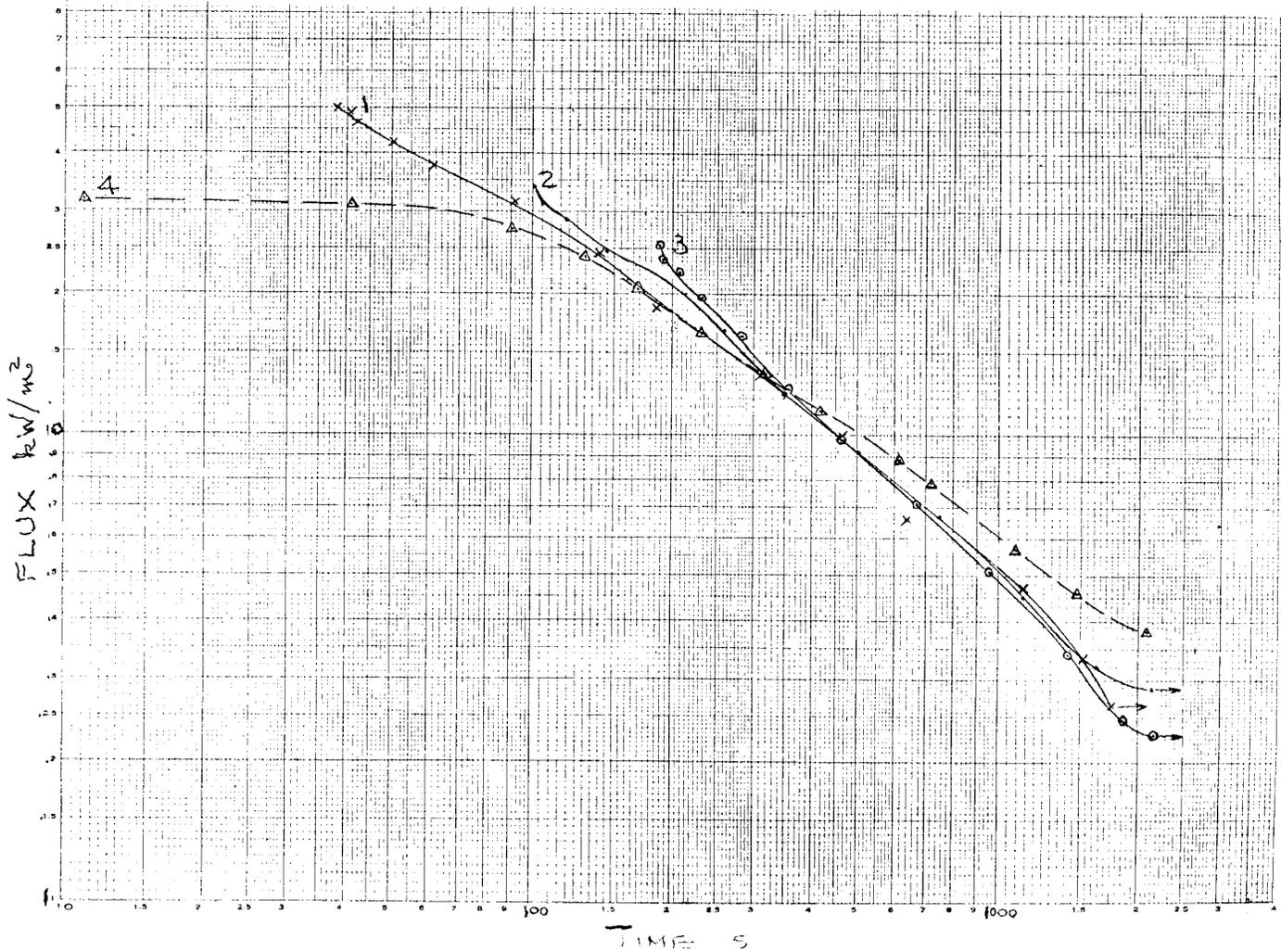
NOTE 1—The dotted line corresponds to the heat for sustained burning of 2.7 MJ/m<sup>2</sup> specified in 12.1.9.3.
