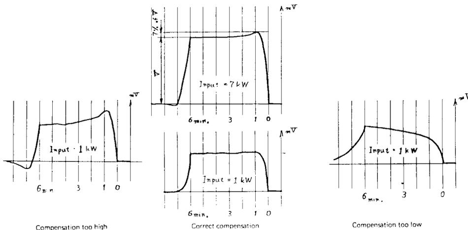
NOTE 1—The four curves shown illustrate changes in the indicated mV signal rise for three different levels of inverse feedback or compensation level.
