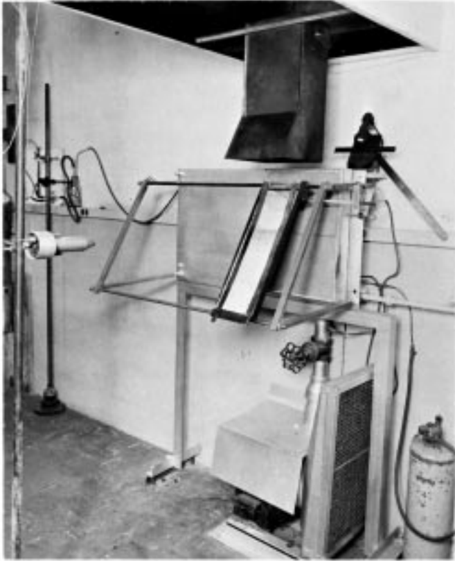
FIG. 1 Radiant Panel Flame Spread Test Equipment
