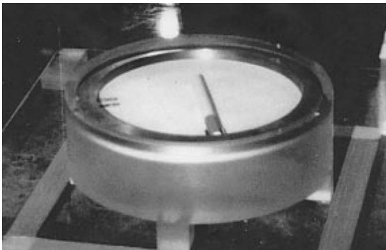
FIG. 2 Close-up of Test Cigarette, Filter Paper Holder, Metal Pins and Metal Rim
