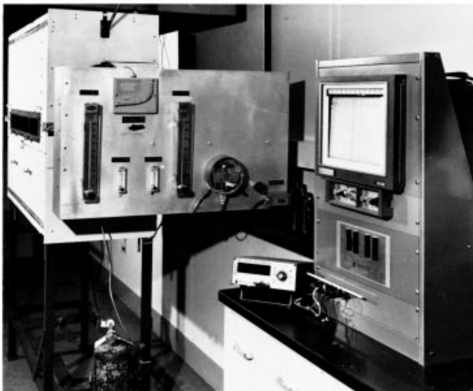
FIG. 1 Flooring Radiant Panel Tester Apparatus
