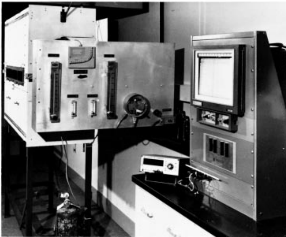
FIG. 1 Flooring Radiant Panel Tester Apparatus
