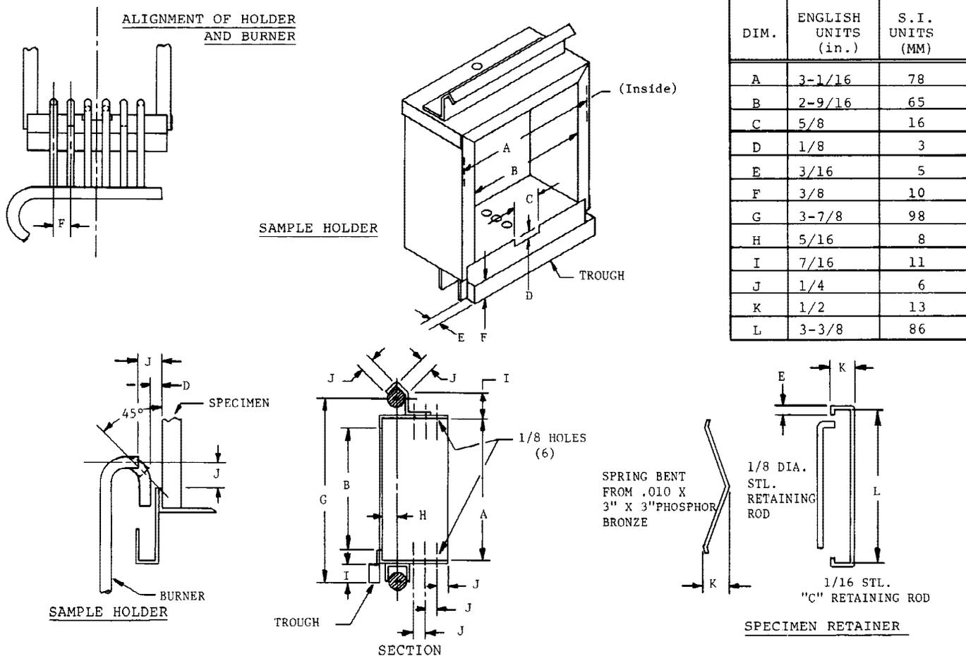
FIG. 4 Details of Specimen Holder and Pilot Burner
