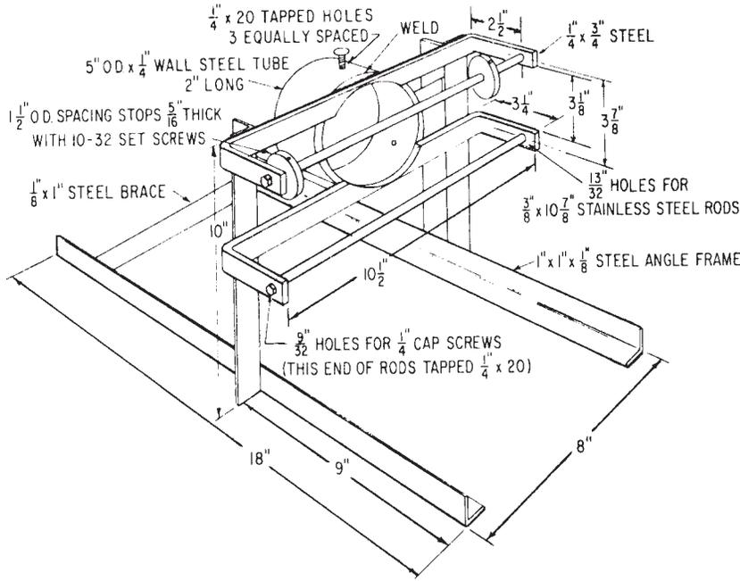
FIG. 5 Furnace Support
