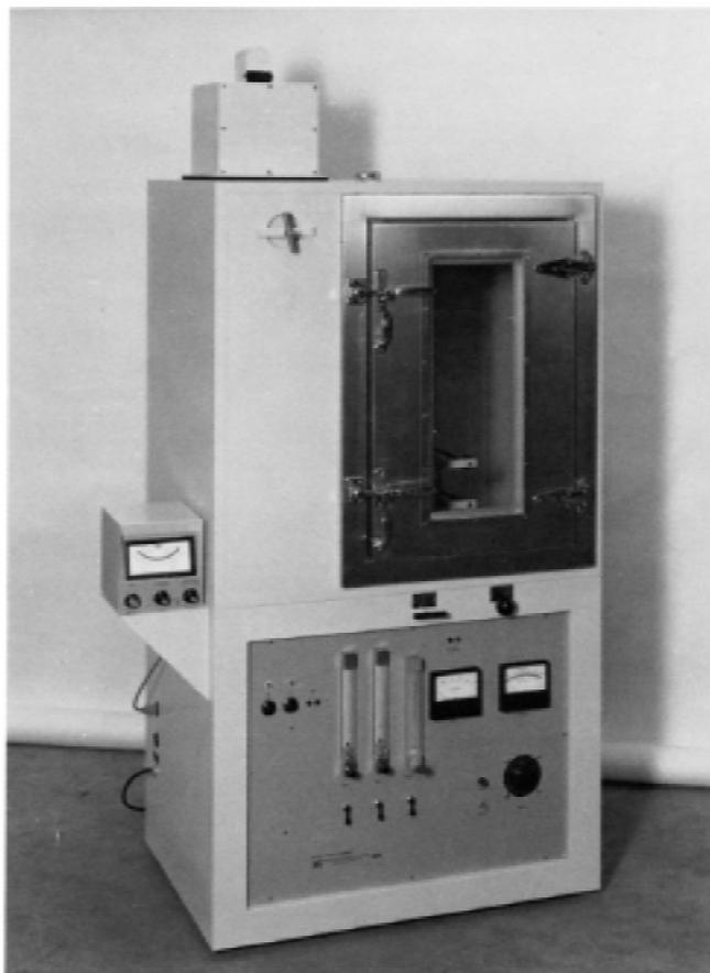
**FIG. 1 Smoke Density Chamber**
