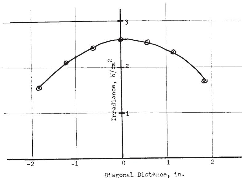
FIG. X4.1 Diagonal Survey of Irradiance at Specimen During Operation at Nominal 2.5 W/cm<sup>2</sup>
