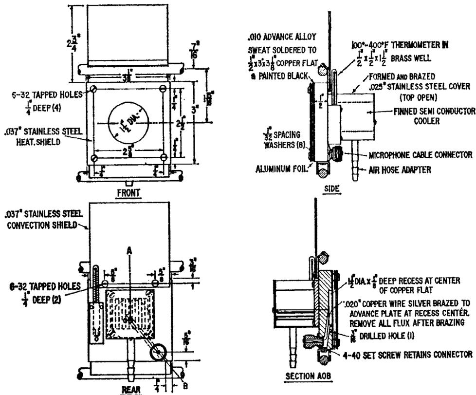
FIG. 8 Radiometer Details
