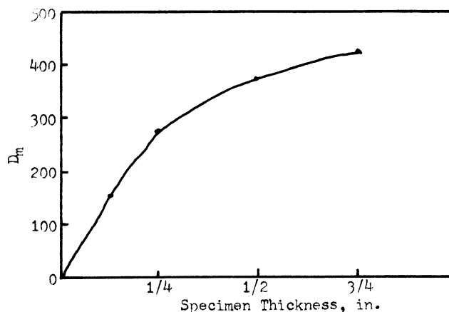
FIG. X4.2 D_m for Spruce as a Function of Specimen Thickness Under Nonflaming Conditions
