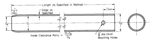
Note 1—Minimum of two mounting holes on opposite sides for  $D_0$  smaller than 4 in. (101.6 mm).
