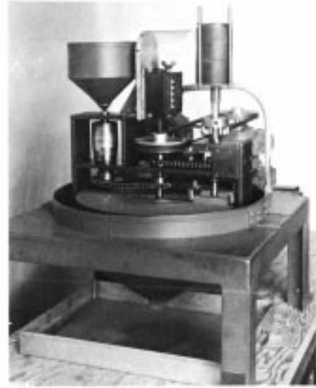
FIG. 20 Navy-Type Wear Machine for Abrasion Resistance Test
