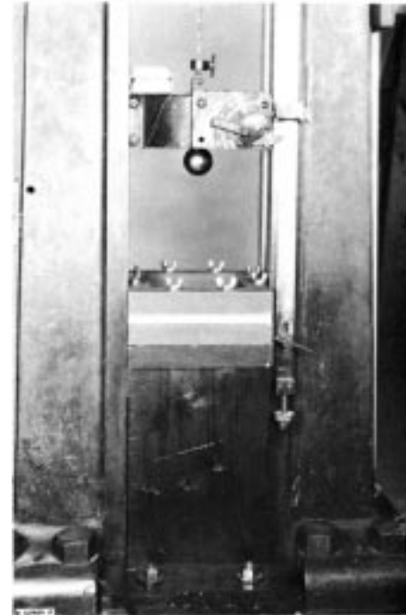
FIG. 18 Test Assembly for Falling Ball Impact Test
