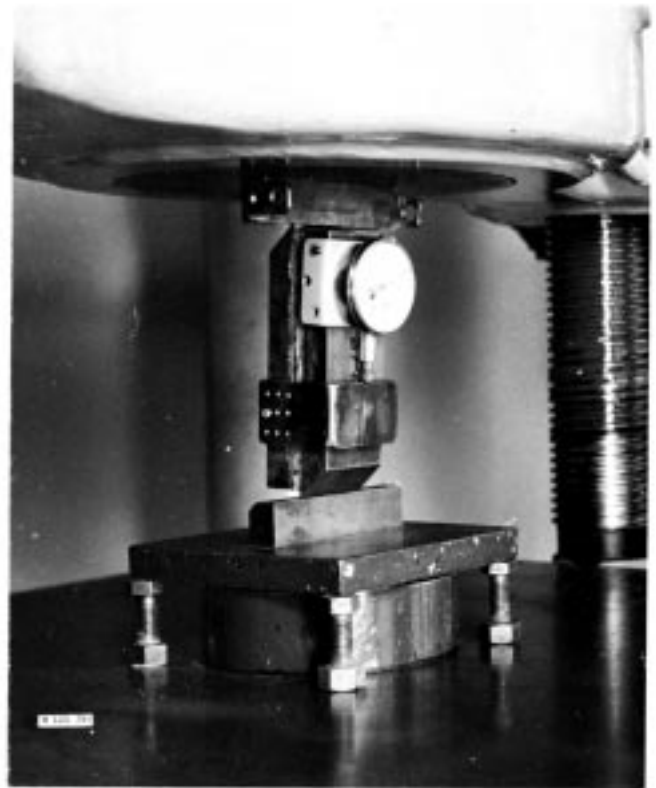
FIG. 27 Test Assembly for Determining Interlaminar Shearing Properties, Showing Dial Gage Apparatus for Measuring Shear Displacement
