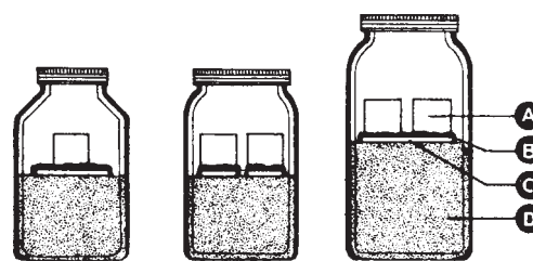
A—Wood cubes, 19-mm or 0.75-in. B—Test fungus growing over feeder block. C—Wood feeder block. D—Soil.
