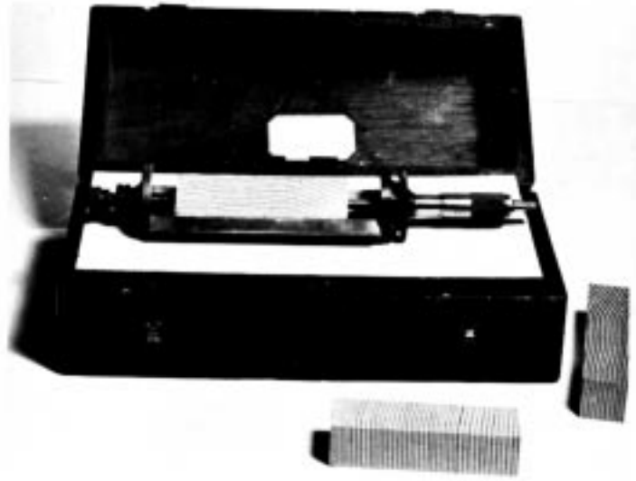
FIG. 41 Radial- and Tangential-Shrinkage Test Assembly
