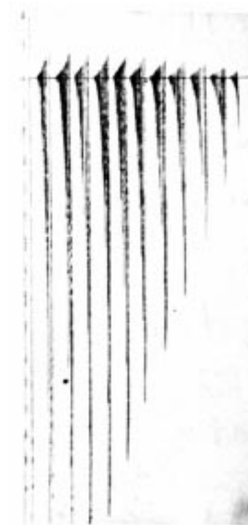
FIG. 12 Sample Drum Record of Impact Bending Test
