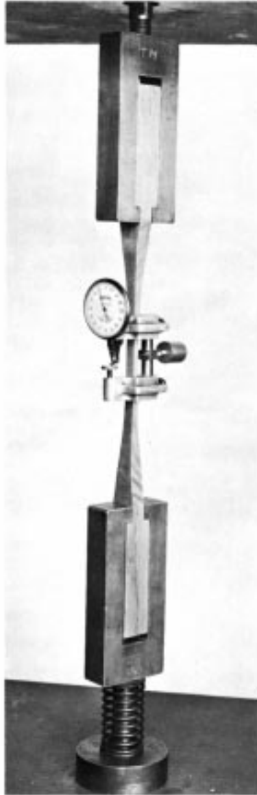
FIG. 29 Tension-Parallel-to-Grain Test Assembly Showing Grips and Use of 2 in. (50-mm) Gage Length Extensometer for Measuring Deformation
