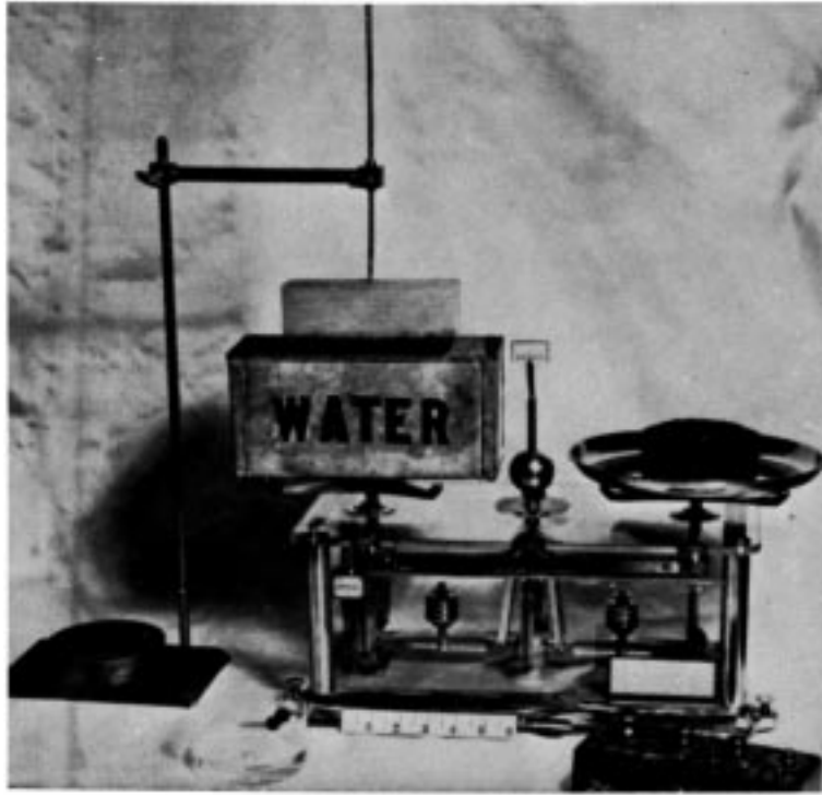
FIG. 39 Specific Gravity and Shrinkage-in-Volume Test Set-Up
