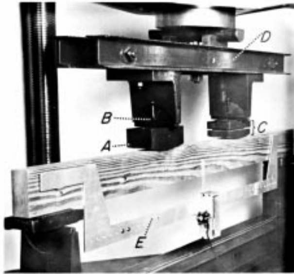
FIG. 4 Example of Curved Loading Block, A, Load-Alignment Rocker, B, Roller-Curved Loading Block, C, Load Evener, D, and Deflection-Measuring Apparatus, E
