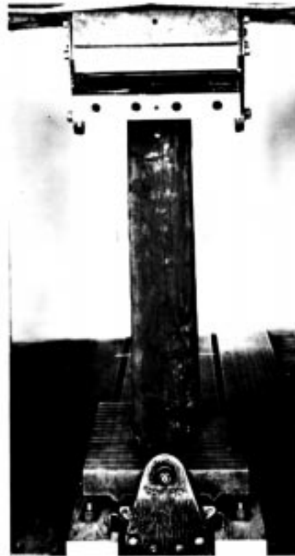
FIG. 5 Compression of a Wood Structural Element
