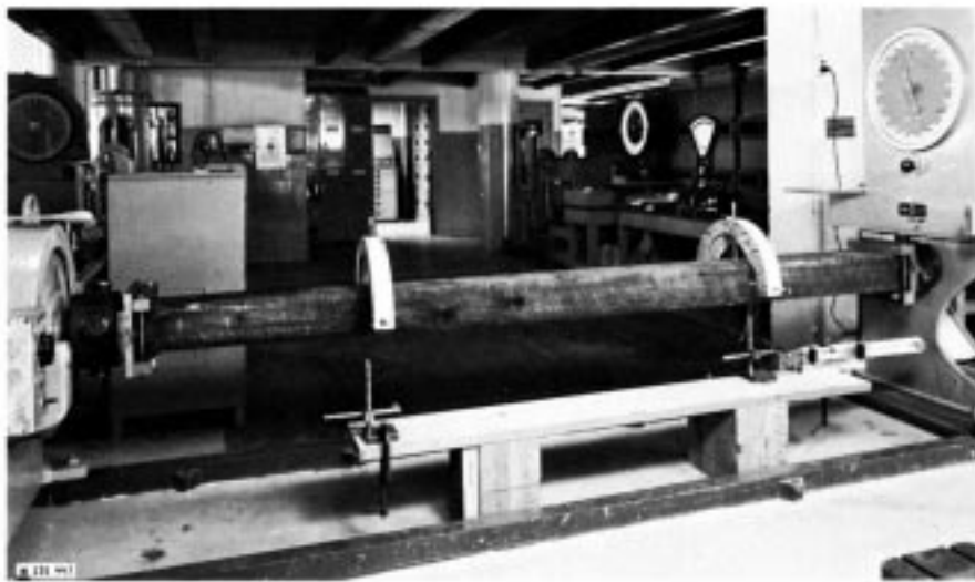
FIG. 15 Torsion Test with Yoke-Type Troptometer
