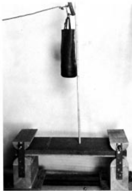
FIG. 6 Apparatus for Impact Load Test, Pictorial
