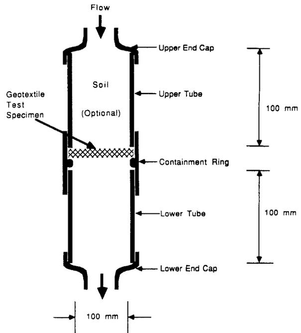
FIG. 1 Flow Column to Contain Geotextile Test Specimen
