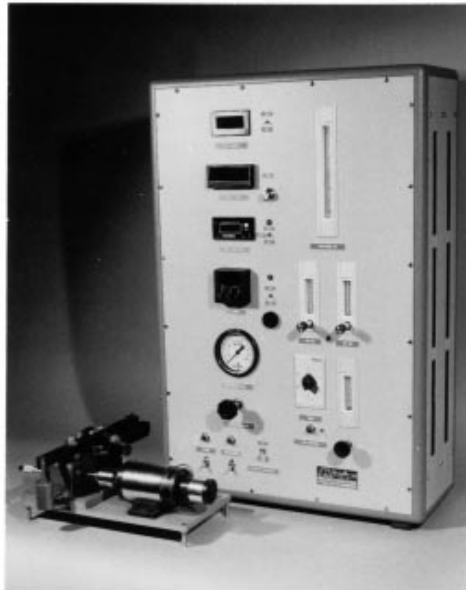
FIG. 1 Ball-on-Cylinder Lubricity Evaluator
