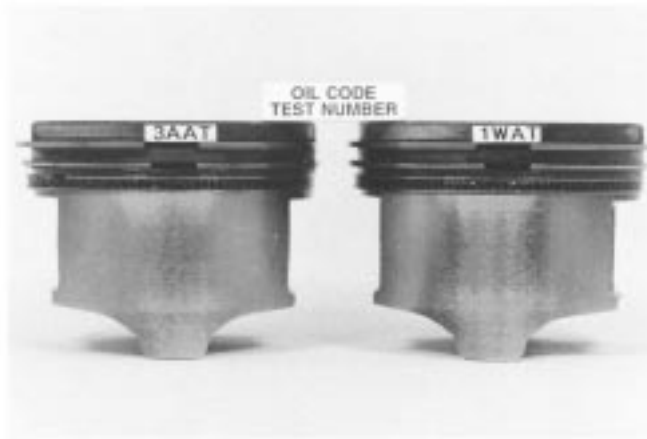
FIG. A7.16 Piston Skirt Photographs
