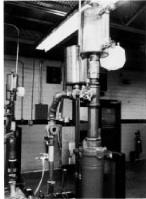
FIG. A3.9 Typical Engine Cooling System, Flow Control Valve, Venturi Flowmeter, Expansion Tank, and Sight Glass
