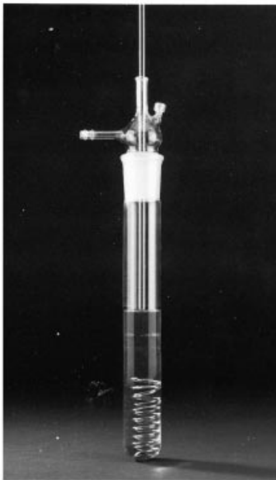
FIG. 3 Assembled Test Cell Ready to Insert Into Heating Block
