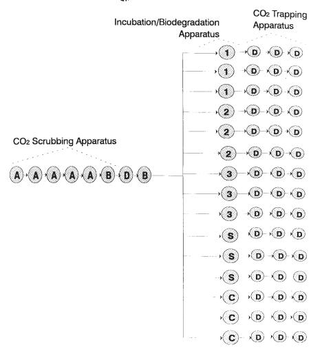
A = NaOH B = Empty C = Blank S = Standard  $D = Ba(OH)_2$  1 = Test substance 12 = Test substance 2
