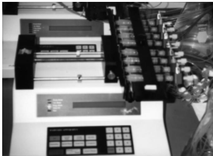
FIG. 3 Photograph of Acid Delivery System
