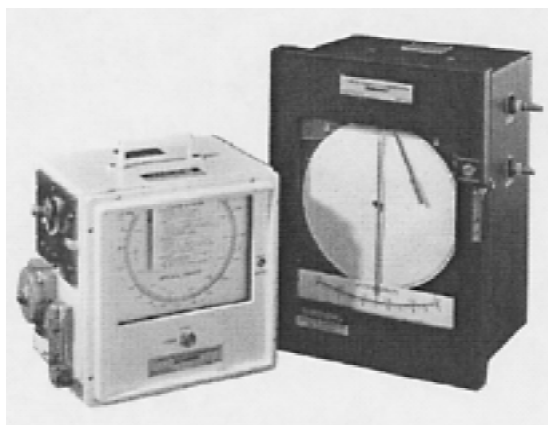
FIG. 1 Examples of Portable and Recording Ranarex Gravimeters.
