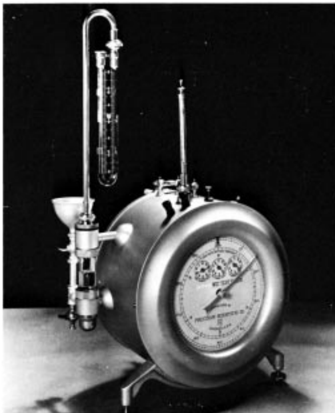
FIG. 3 Liquid-Sealed Rotating-Drum Gas Meter of 0.1 ft 3 per Revolution Size
