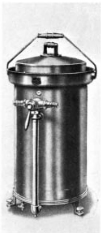
FIG. 1 Stillman-Type Portable Cubic-Foot Standard
