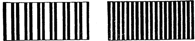
FIG. 4 Stroboscopic Lines Appearing as Multiples that May be Observed Before 200-r/min Reached
