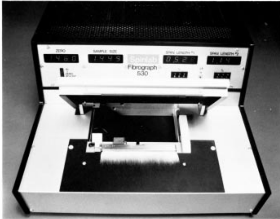
FIG. 1 Digital Fibrograph, Model 530
