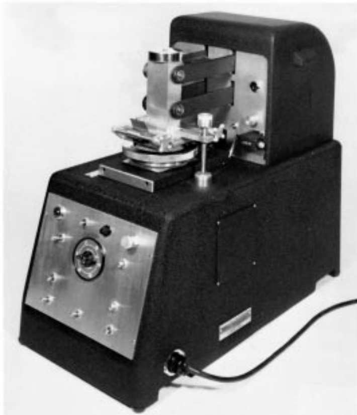
FIG. 2 One Type of Commercial Inflated Diaphragm Abrasion Tester
