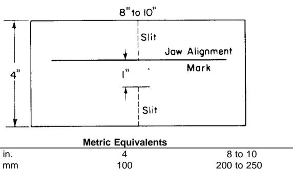
FIG. 1 Illustration of Modified Grab Test Specimens
